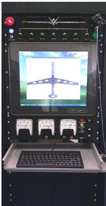
US Navy BAMS/TRITON DE-ICING SYSTEM ATE
